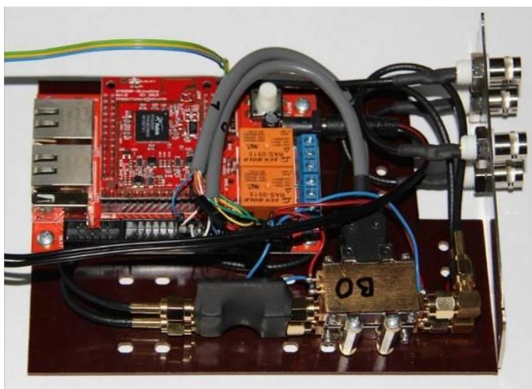
Fig. 3 Prototype of remotely controlled attenuator
