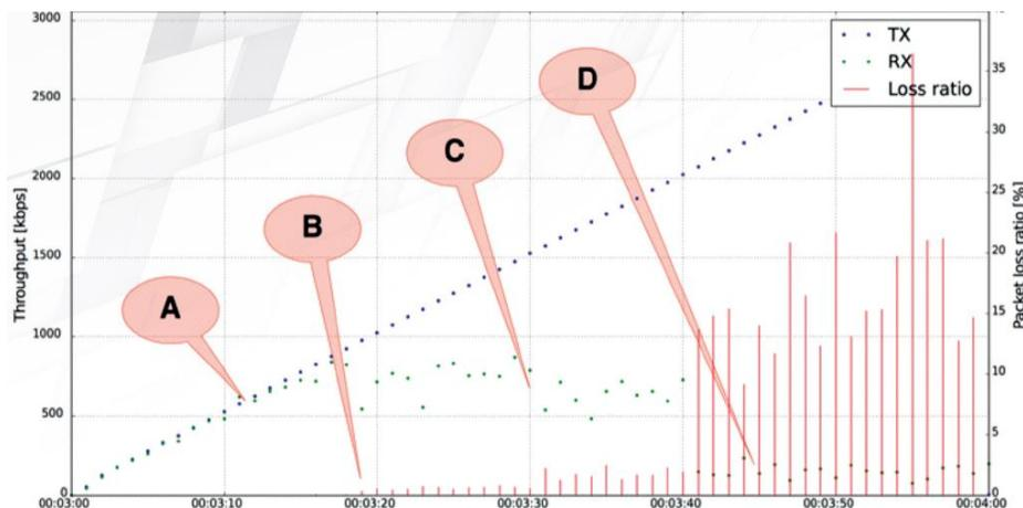
Fig. 6 Data throughput measurement – ramp test
