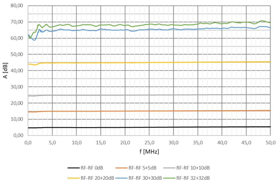
Fig. 4 Frequency dependence of attenuation for different settings
