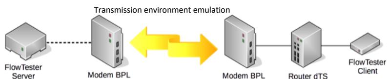
Fig. 1 Basic principle of BPL modems testing
